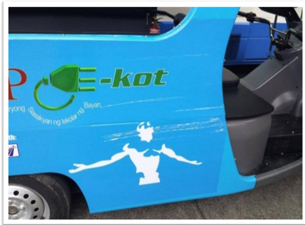
Figure 6. Side of the E-trike Sideswept by a Public Utility Jeepney at Osmeña Avenue
