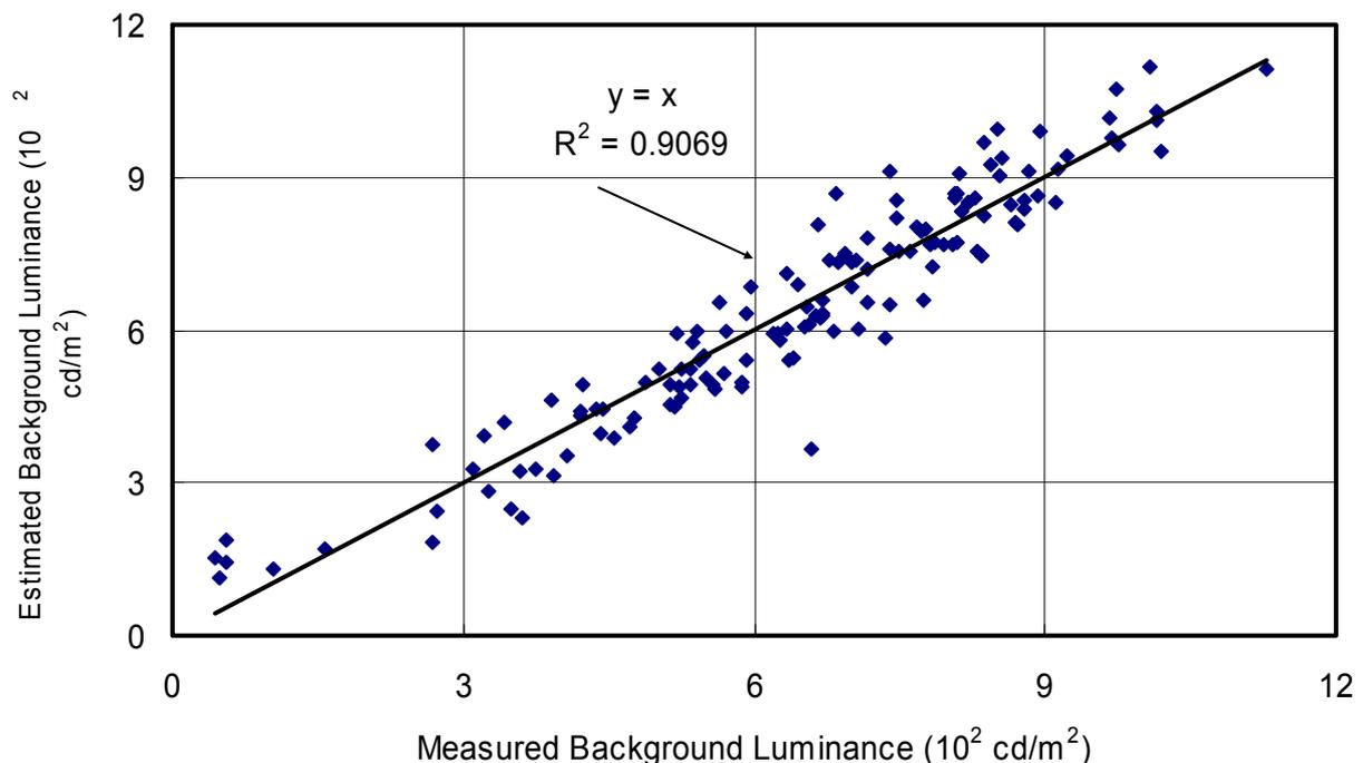
Figure 6 Correlation between measured background luminance and estimated background luminance by the multi-linear regression model in daytime fog.
