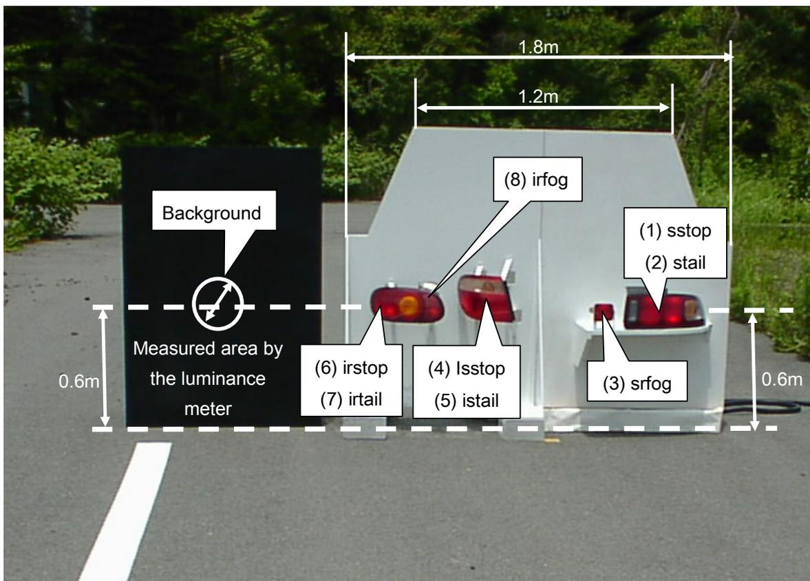
Figure 1. Configuration of eight rear lamps and backgrounds.
