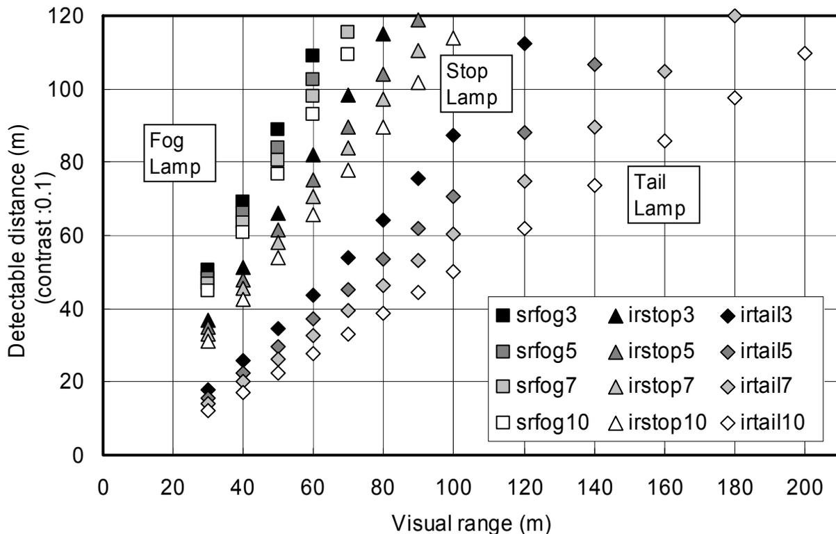
Figure 9 Effect of illuminance conditions on detectable distance as a function of visual range.
