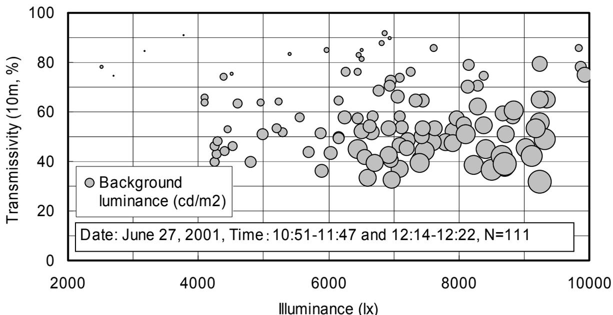
Figure 4 Scatter plot diagram of transmissivity at 10 m, illuminance and background luminance.
