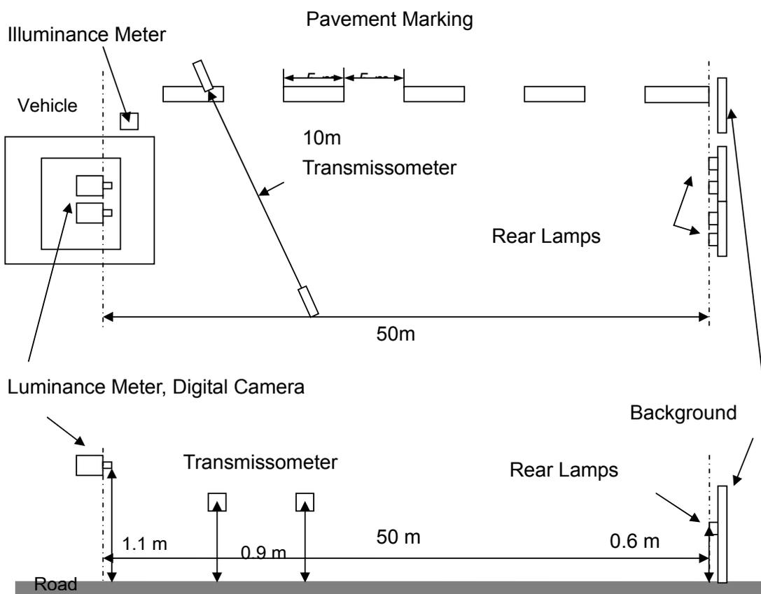
Figure 2. Location of measurement devices at experiment site.
