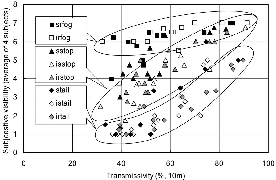
Figure 5 Subjective visibility assessment value versus transmissivity at 10 m as a function of the eight rear lamps.
