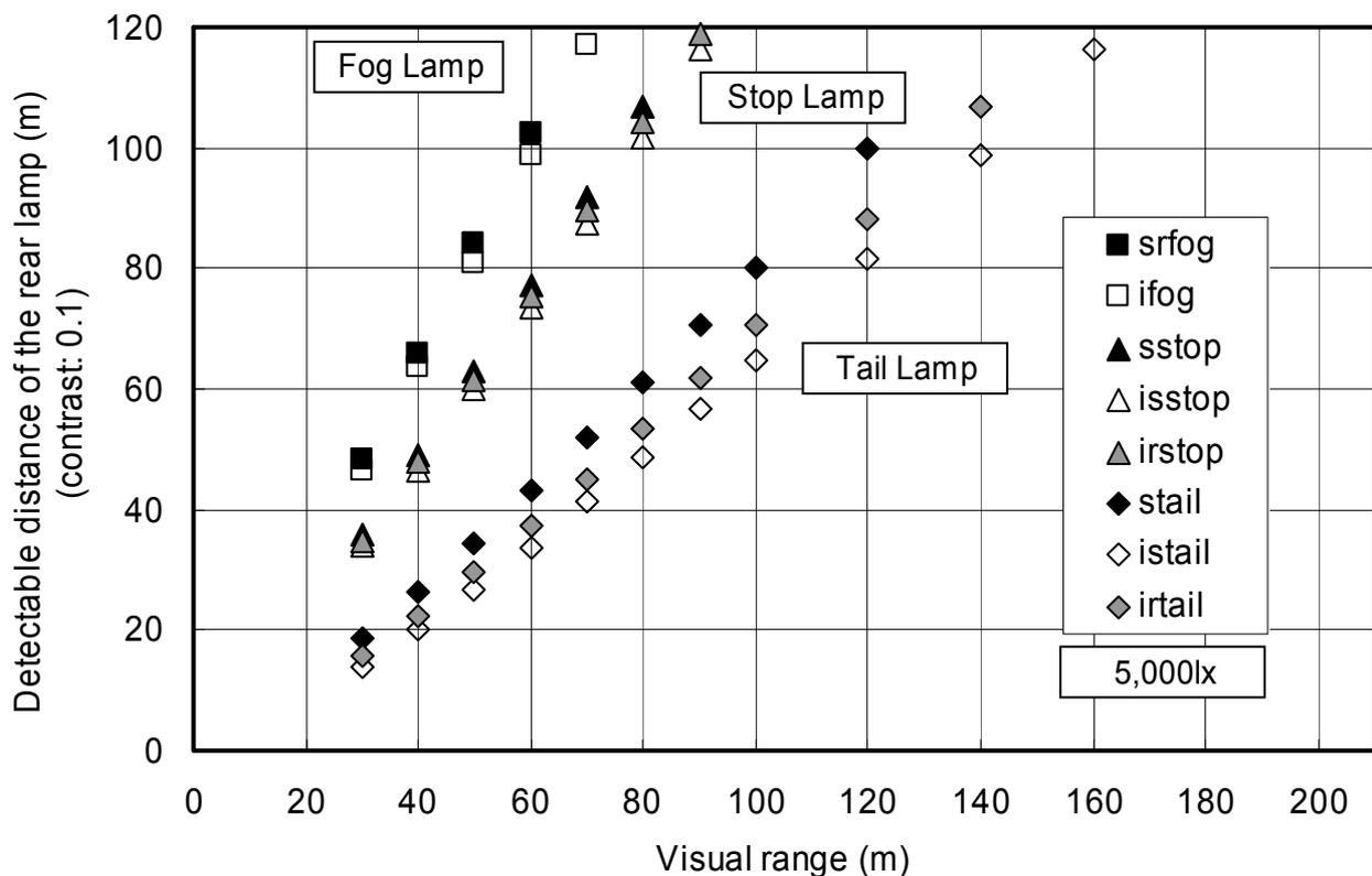
Figure 8 Visual range versus detectable distance calculated by equation (2) when contrast of the rear lamp is 0.1. (visual range: 30 m to 200 m, illuminance: 5,000 lx)
