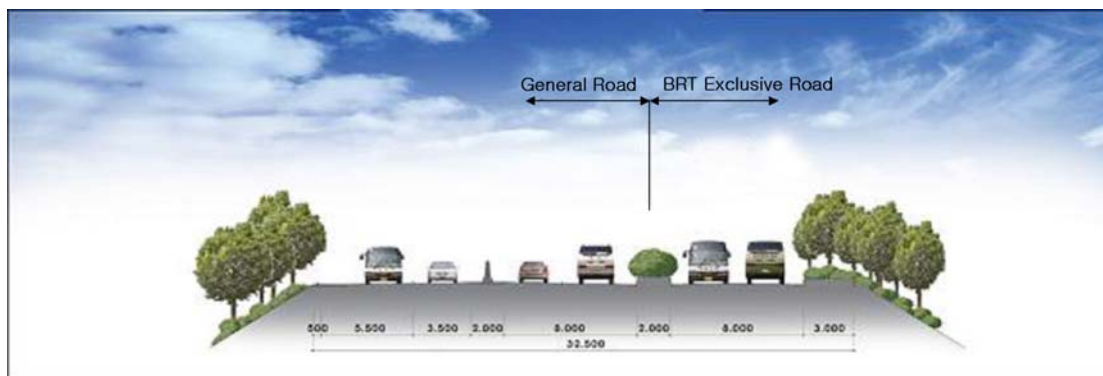
Figure 7. Cross Section View of An Exclusive BRT Road Along With General Road
