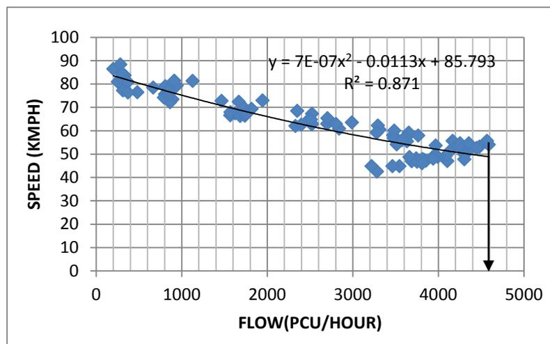
**Figure 16. Speed–Flow curve in terms of PCE per hour**
