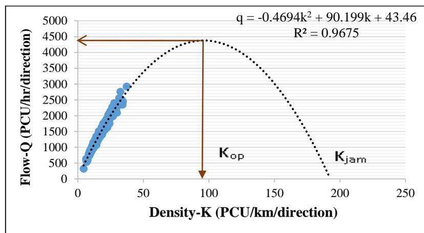
**Figure 10 Flow-Density Curve**
