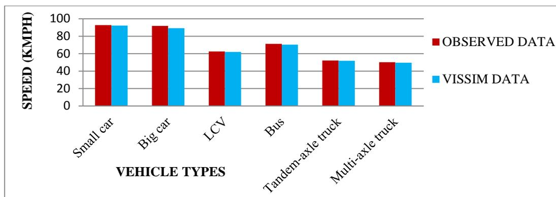
Figure 13 Comparison of field observed mean speeds and VISSIM mean speed
