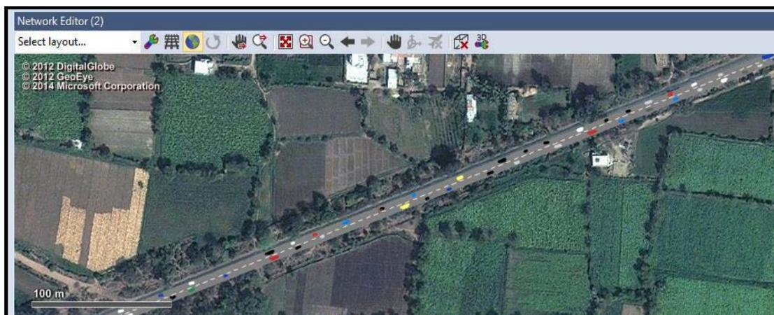
Figure 12 Snapshot of simulation runs in VISSIM with reference to location
