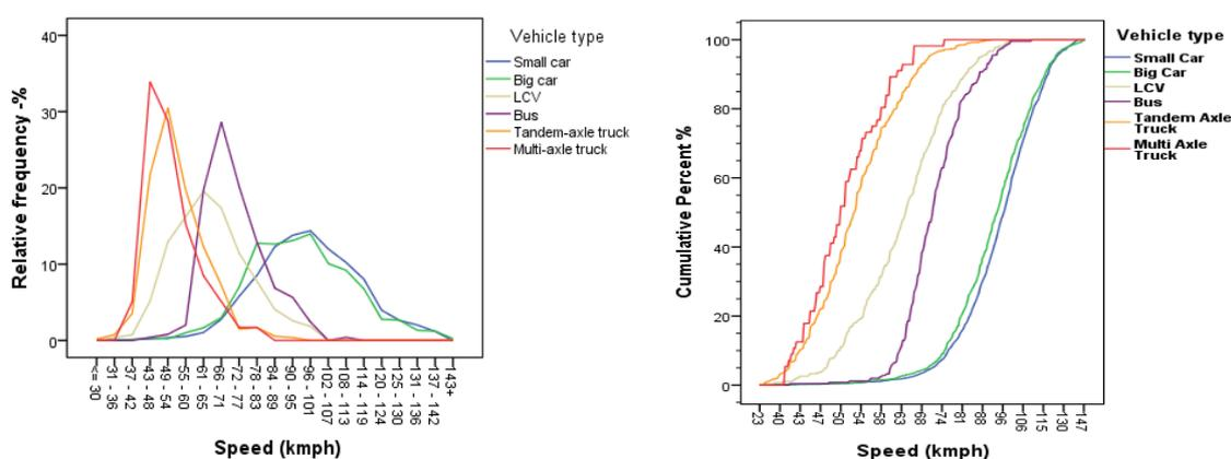
Figure 7 (a) Relative Frequency distribution of speed; (b) Cumulative plot of speed
