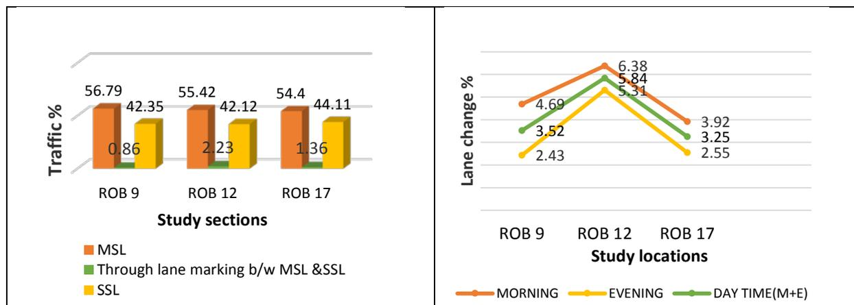
**Figure 6 (a) Vehicle distribution over carriageway; (b) Lane changes on different sections**
