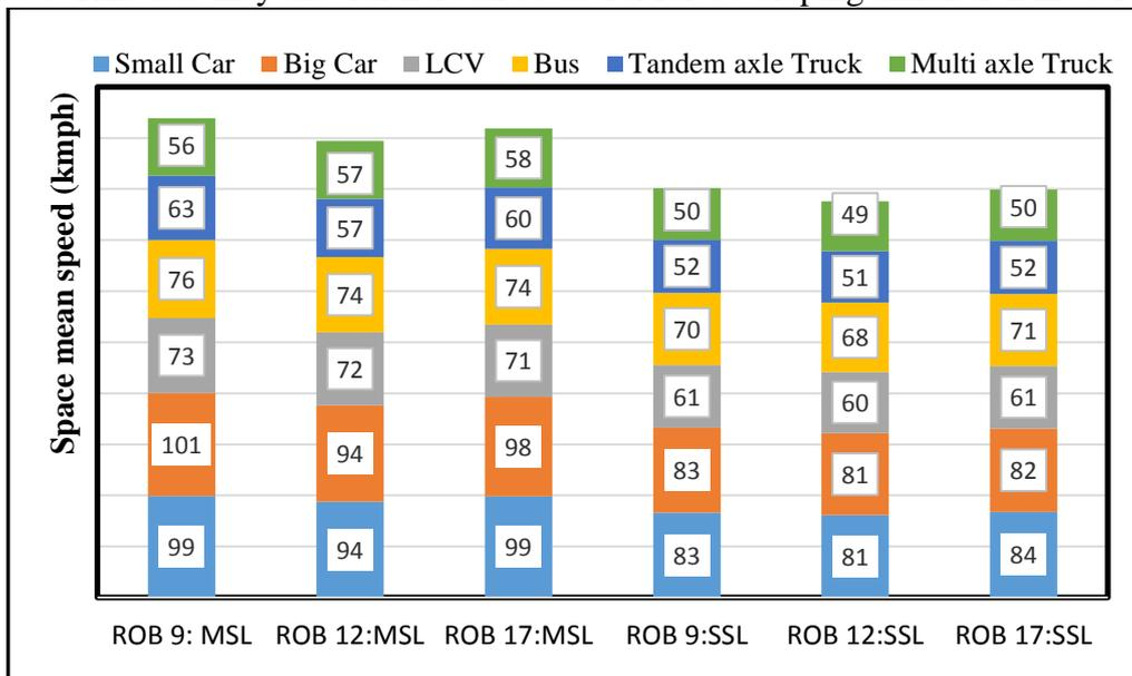
**Figure 8 Lane wise space mean speed of different vehicles on different sections**
