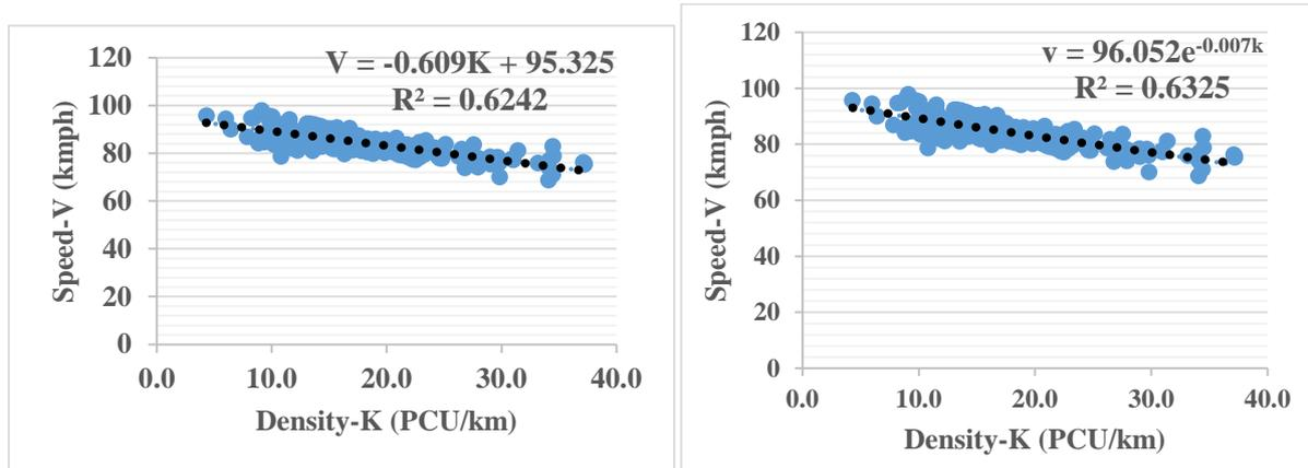
**Figure 9 Speed-Density Curve**
