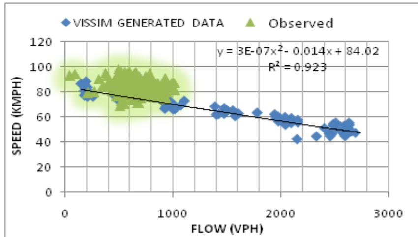
Figure 14 Speed – Flow curve in terms of vehicles per hour
