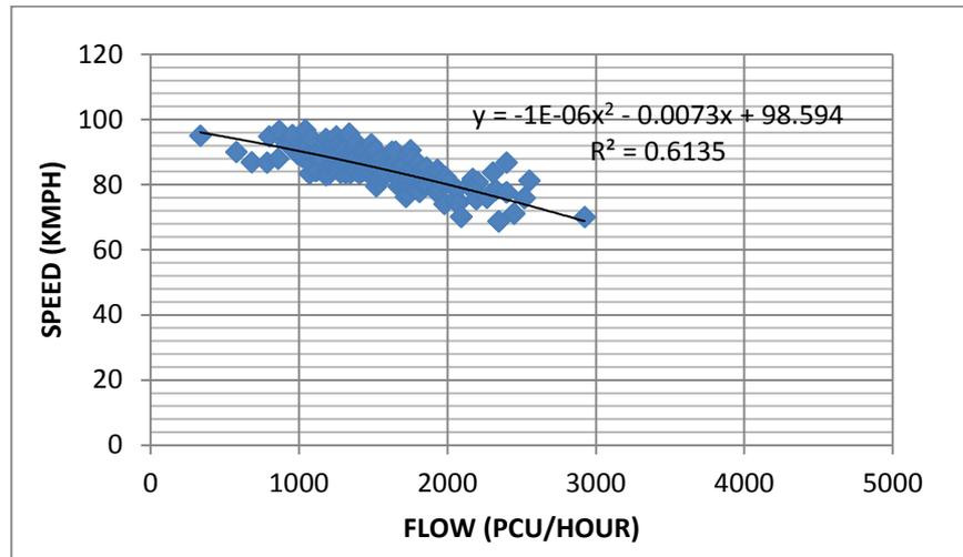
**Figure 11 Speed- Flow Curve**
