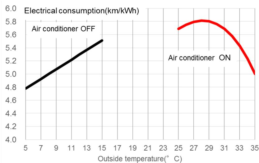
Figure 11. The relationship between EV's electrical consumption and average outside temperature
