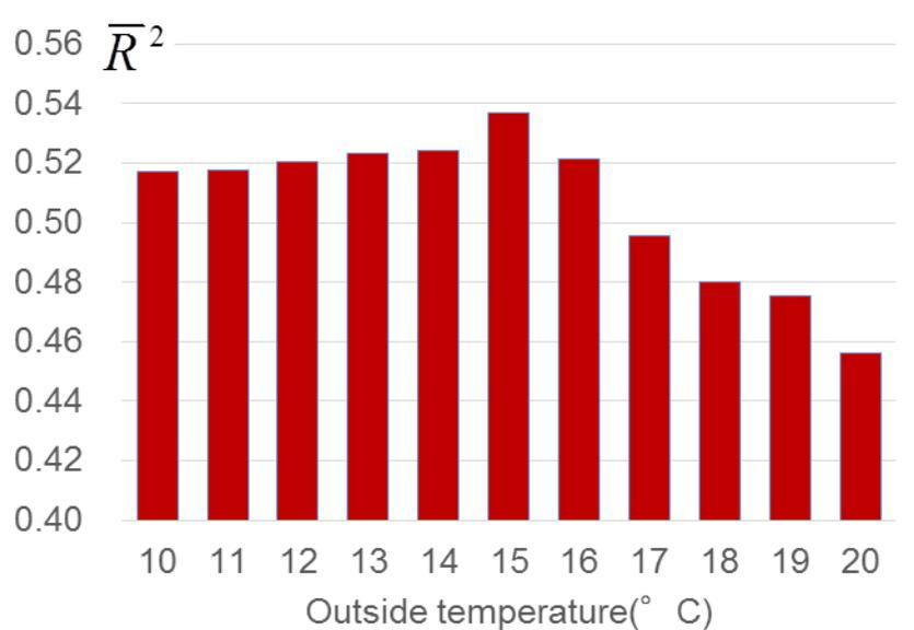
Figure 10. The coefficient of determination by threshold of outside temperature
