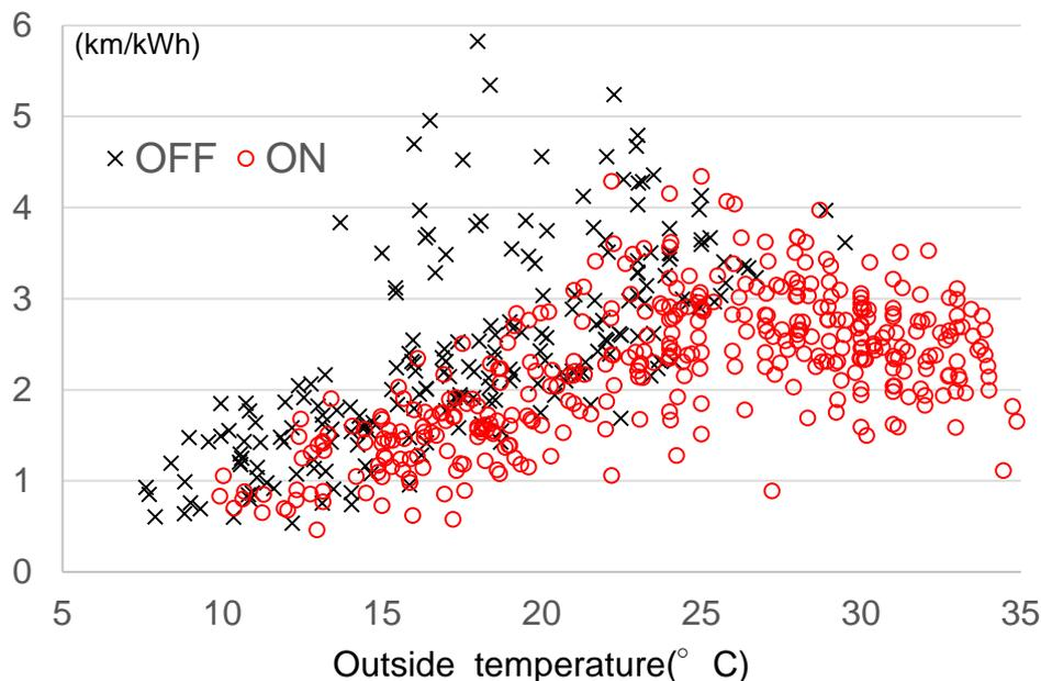
Figure 9. Scatter plot of relationship of EV's electrical consumption and air conditioner usage (o: air conditioner ON; x: air conditioner OFF)
