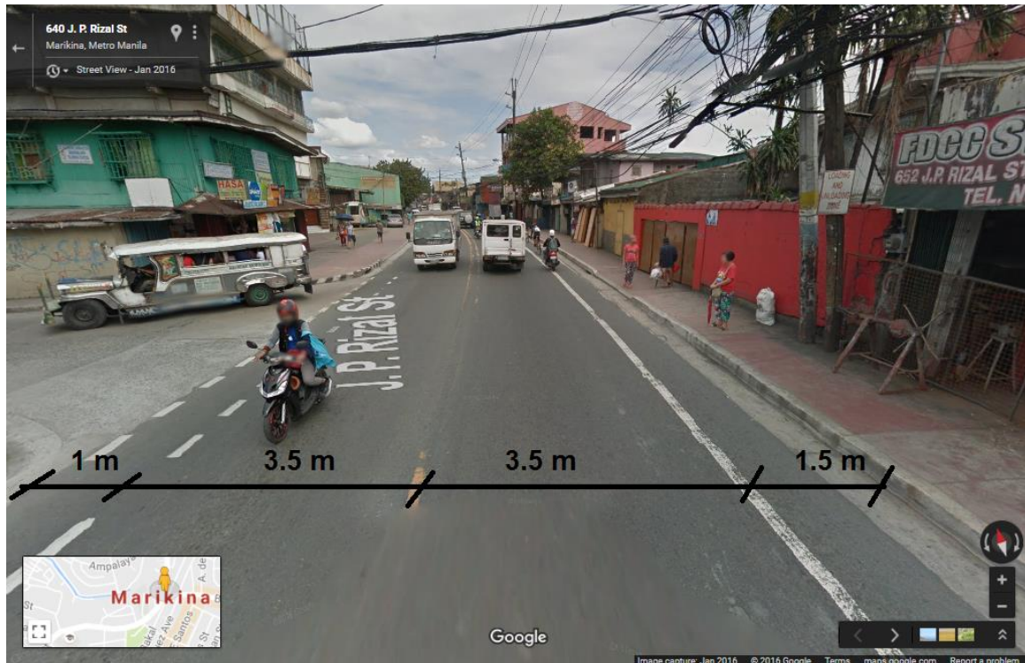
Existing Road Width Dimension
