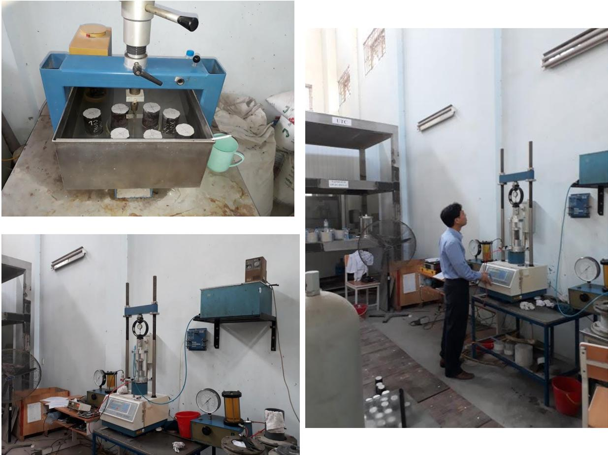
Figure 9. Triaxial test for FAM
