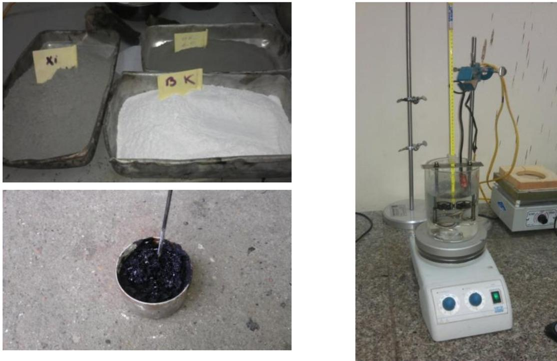
Figure 6. The ring and ball test for softening point of the bitumen and the mastic asphalt
