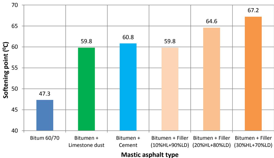
Figure 5. The softening point of the bitumen and the mastic asphalt types
