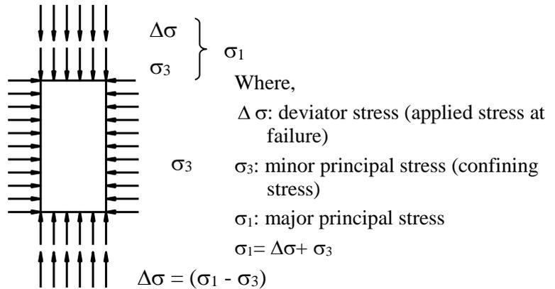
Figure 3b. The stress state in the triaxial test
