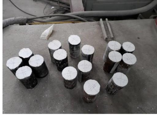
Figure 2. FAM specimens for triaxial test
