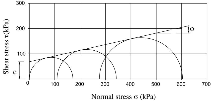
Figure 4. Mohr circles and Mohr-Coulomb failure envelope
