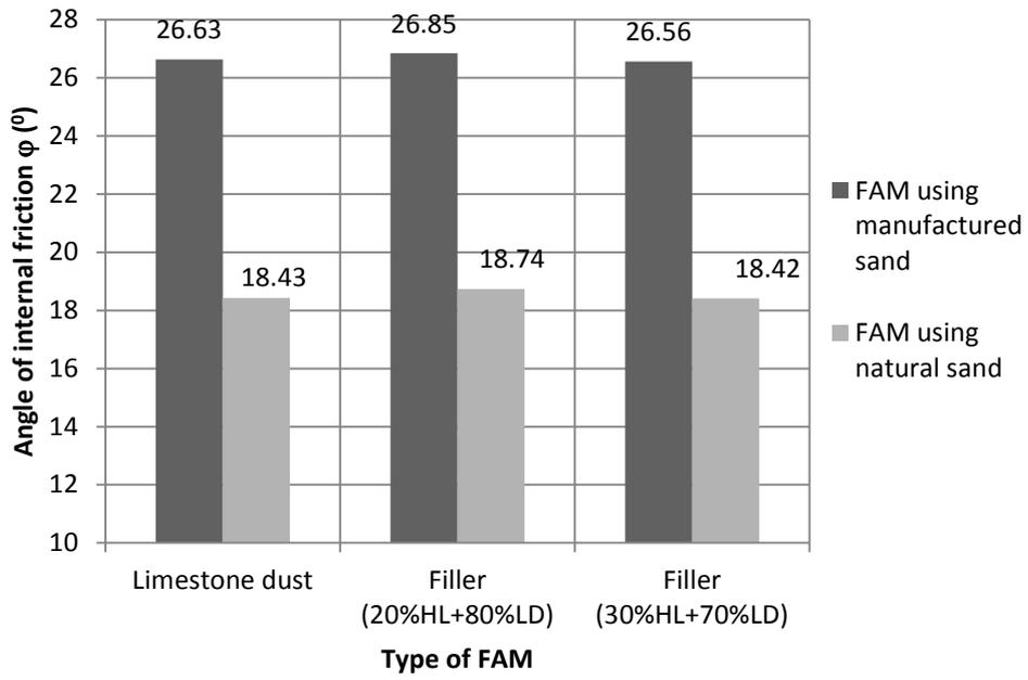
Figure 7. The internal friction angle of FAM at 30°C
