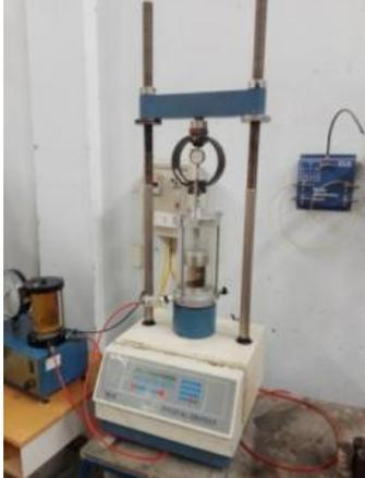
Figure 3a. Triaxial apparatus
