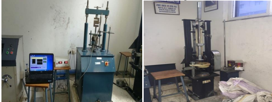
Figure 3 Marshal setup – Online DAQ with automatic compactor
