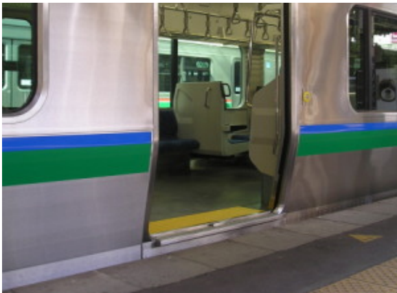
Photo 5: Less difference in level between platforms and floors of vehicles
