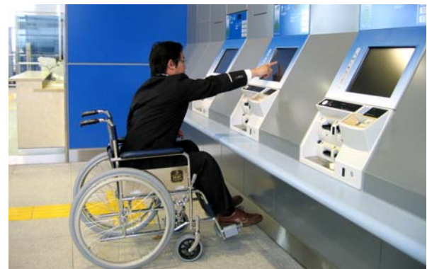
Photo 4: The train ticket vending machine that considered height and a slant
